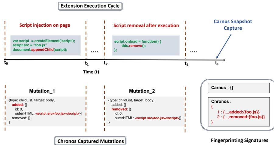
Figure 2: Extension execution timeline and continuous fingerprint generation.
