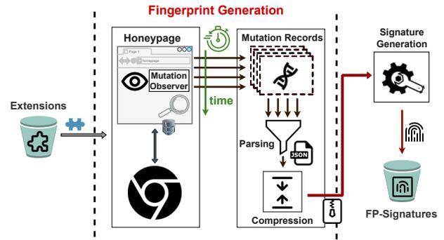
**Figure 1: High level representation of our system Chronos.**
