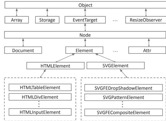
Figure 6: Inheritance hierarchy in the DOM API.
